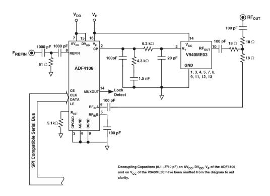
Figure 3. The ADF4106 used to implement a 6.0-GHz local oscillator.
