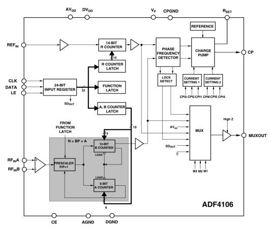
Figure 1. Functional block diagram of the ADF4106
