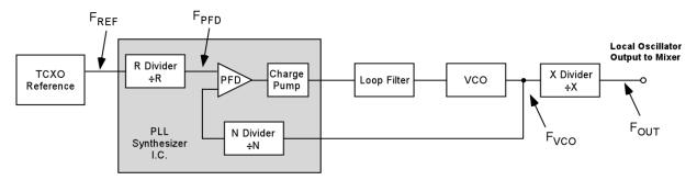
Figure 4. Architecture for improved lock time, phase noise and reference spurs.
