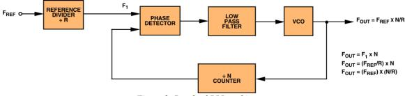
Figure 2. Standard PLL architecture
