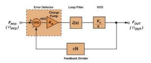
Figure 7. Basic phase-locked-loop model.
