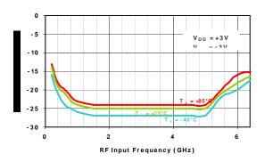
Figure 6. ADF4106 sensitivity vs. frequency.
